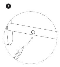
Hold the rod against the wall, make sure it is leveled. Use the two holes to mark where to drill. After drilling, insert adequate wall plugs suited for you wall type.
