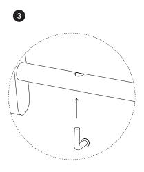
Slide the coat rack down onto the L-hooks.
