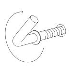
Screw the L-hooks into the wall. Continue screwing until the discs cover the plugs.
